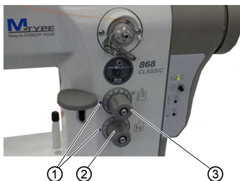
Fig. 49: Setting the stitch length
