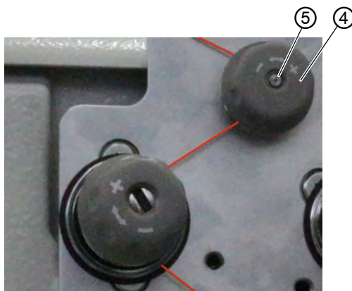
Fig. 31: Setting the needle thread tension (2)
