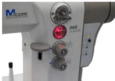
Fig. 66: Checking the oil level (2)
