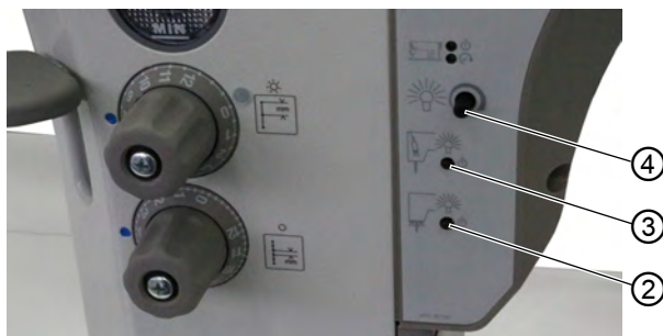
Fig. 5: Switching on and off the sewing lamp (2)
