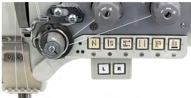
Fig. 61: Assigning functions to buttons on the push button panel
