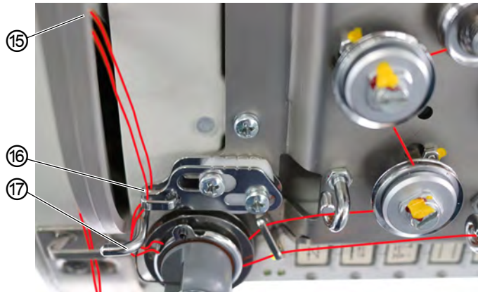
(15) - Thread lever (not visible) (17) - Hook (16) - Needle thread regulator
