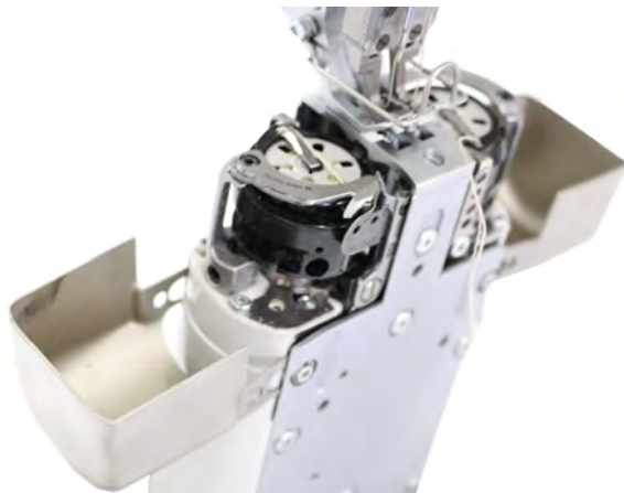
Fig. 22: Changing the left bobbin (2-needle machine)
