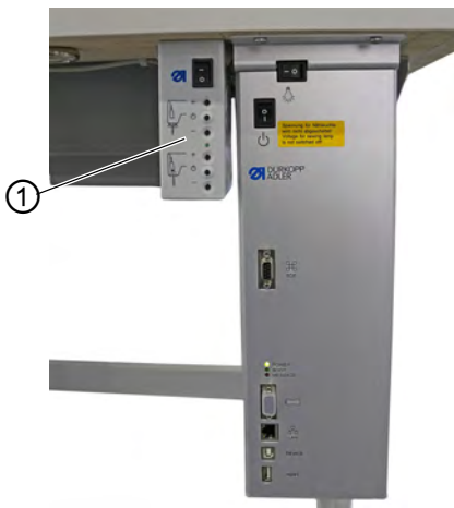
(1) - Sewing lamp transformer
