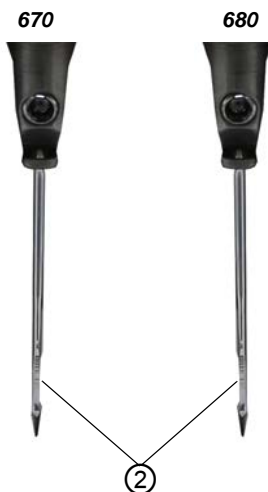
Fig. 6: Changing the needle (2)
