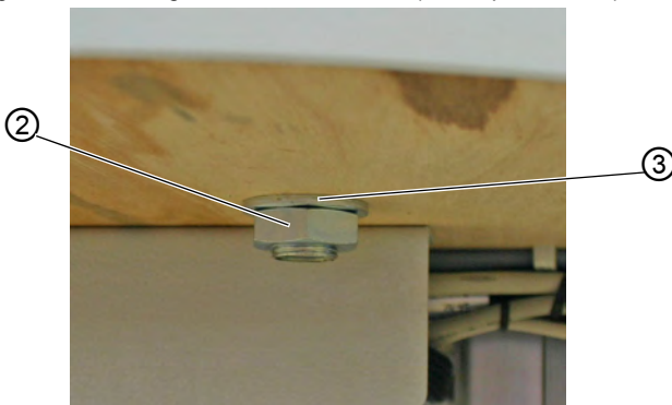
Fig. 58: Assembling the thread reel holder (tabletop underside)
