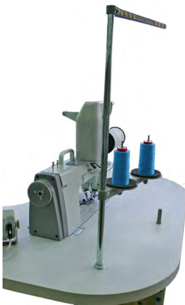
Fig. 56: Assembling the thread reel holder (final state)
