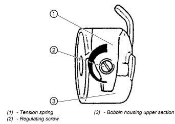
The required hook thread tension must be generated by the tensioning spring (1). The bobbin housing upper section (3) should slowly fall under its own weight when held by the threaded hook thread.
