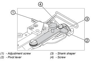
The button clamp can be optionally equipped with a shank shaper (3).
