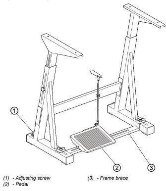
Assemble the individual parts of the frame:
