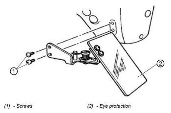
1. Screw the eye protection (2) to the upper section using 2 screws (1).
