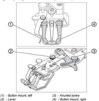
Fig. 9: Adjusting the button mount – optional clamp
