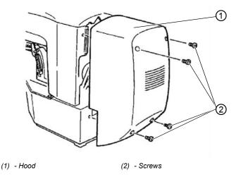
1. Screw the hood (1) to the upper section using 4 screws (2).
