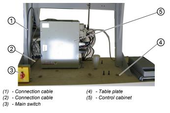
Fig. 24: Completing the table plate (1)
