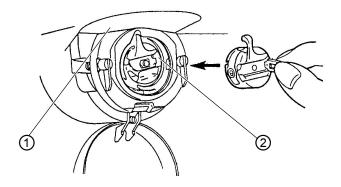
(1) - Underside of throat plate (2) - Hook
