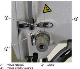
The thread regulator (1) regulates the amount of needle thread required for forming the stitch. An optimum sewing result is only possible when the thread regulator is exactly adjusted.
