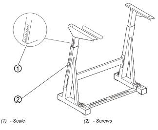
The working height can be adjusted between 750 mm and 950 mm (measured to the upper edge of the table plate). The frame height should correspond to the physical characteristics of the operating personnel.
