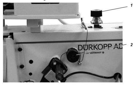
Set the upper needle thread tension by turning the knurled screw 1 and the lower needle thread tension by turning the knurled screw 2.
