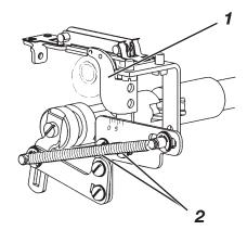
After loosening the screws 2 and adjusting the feeder 1 please make the following settings:
