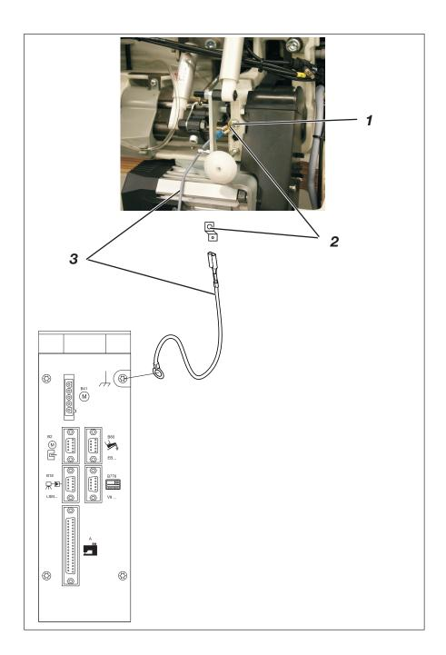
The earthing wire on the sewing machine head bleeds off static charges of the machine head via the motor control unit to the mass.
