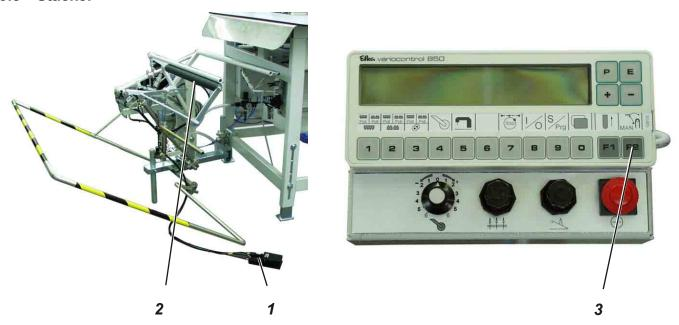
The finished workpieces are stacked on the throw-over stacker 2.
