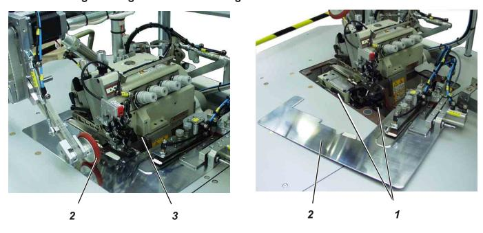
The fabric sliding sheet 2 is held in the gap of the table top by the magnets 1.
