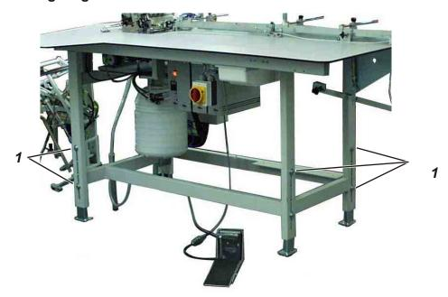
The working height is adjustable between 850 and 1200 mm (measured up to the top edge of the table top).
