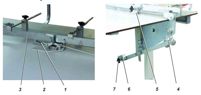
The mouse is used for clamping the trousers and skirt parts to avoid their sliding away.
