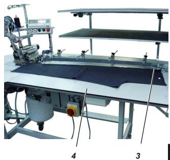
The sewing unit is equipped with two preparation tables 1 and 2. The skirt parts or trousers parts are positioned on them.
