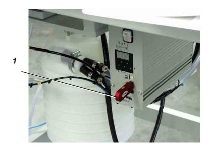
The USB stick 1 serves for storing and transferring of the sewing unit software.
