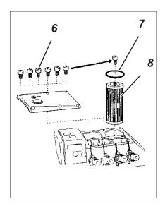
4 weeks after the initial start-up and subsequently every two years an oil change has to be carried out with the machine head disassembled.
