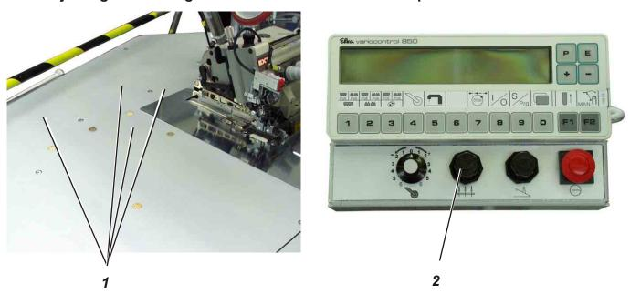
The blowing nozzles 1 in the table top support the precise stacking of the workpieces.
