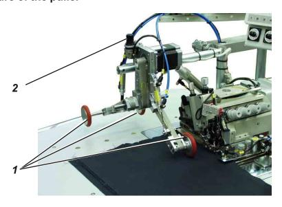
The pressure of the puller rollers 1 can be influenced via turning knob 2.
