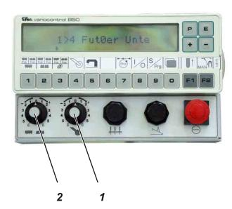
Needle feed, bottom feed and puller feed can be adapted to the sewing conditions with the dials 1 and 2.
