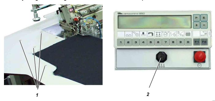
The blast nozzles 1 in the table top support the precise stacking of the workpieces.
