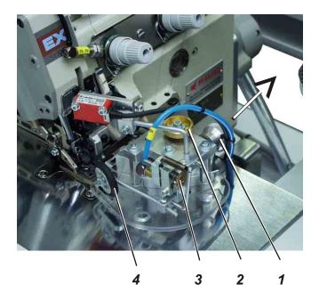
The height-adjustable edge guide ensures a precise positioning of the trousers part in front of the sewing head. The height of the edge guide can be adjusted depending on the thickness of the material to be processed.
