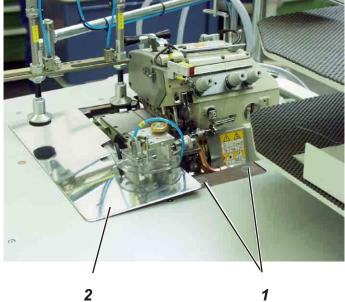
The fabric sliding sheet 2 is held in the gap of the table top by the magnets 1.
